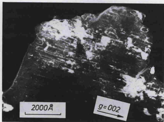
Fig. 2. Dislocations in shocked olivine from Apollo 11 (10085,26). Transmission electron micrograph. Dark field image produced by a reflection \vec{g} = 002 . Particle normal near [010]. Acceleration voltage 100 kV. (Siemens Elmicope 101.)
